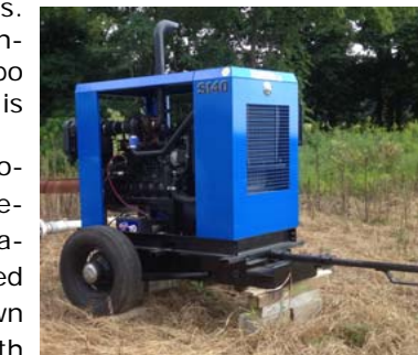
New diesel irrigation engine
