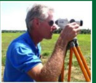
Surveying for the installation of a grassed waterway on a farm in Amagansett is a typical part of the design application.
