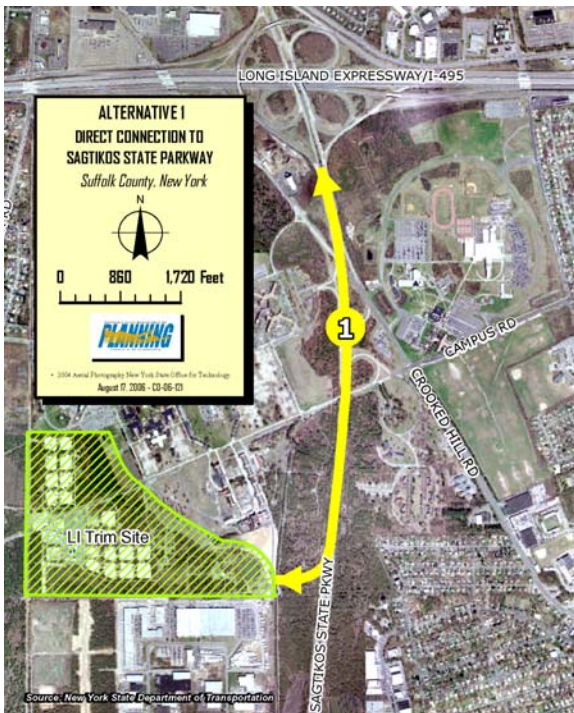
Figure 9. Direct Connection to the Sagtikos State Parkway from the Proposed Truck Rail Intermodal Facility.
